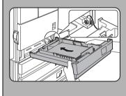
After pulling out the paper tray until it stops, gently lift and pull the tray to remove it. To reinstall the paper tray, insert it at an angle and then push it into the machine.
